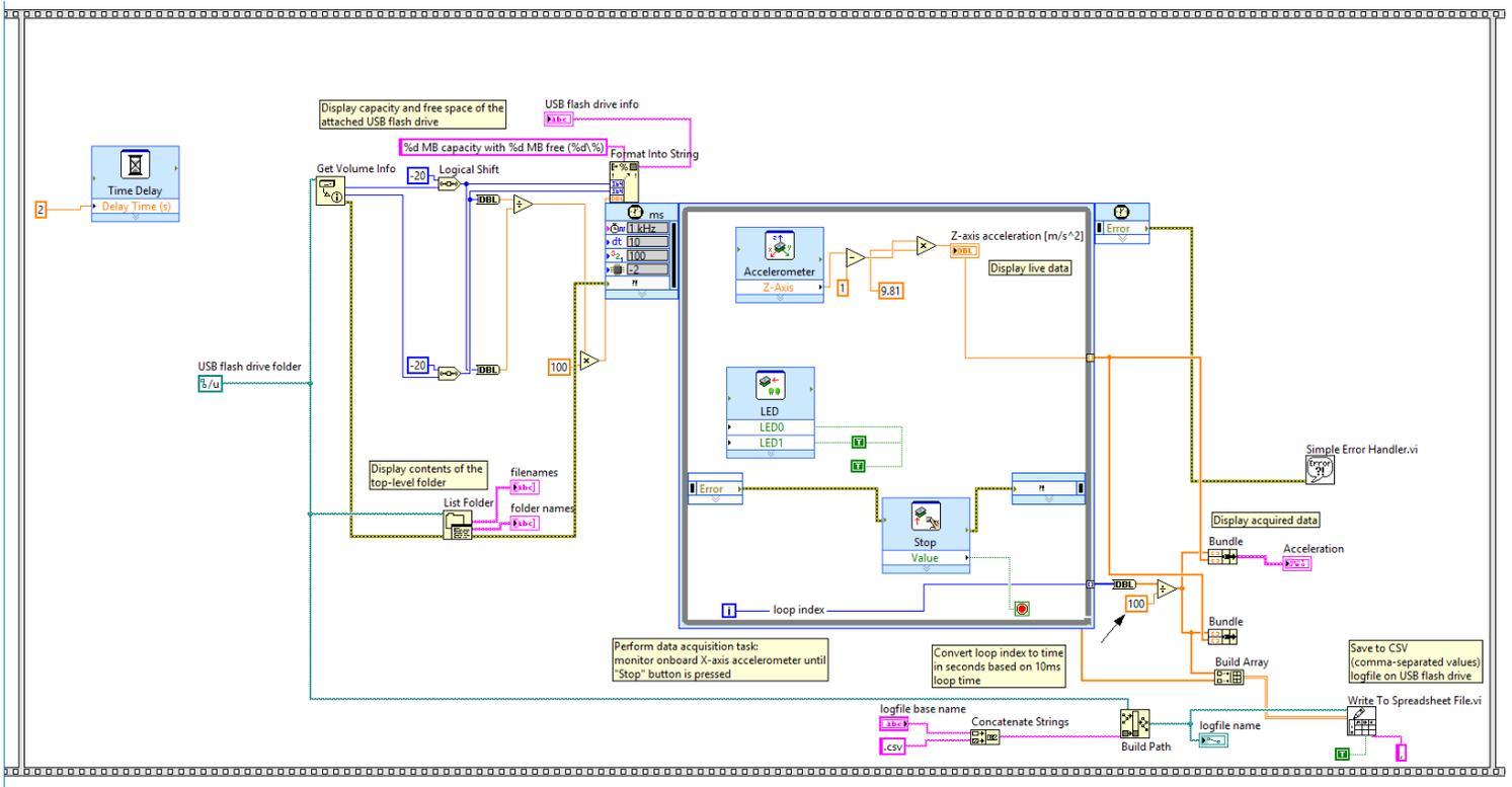
Figure 1. Block diagram z-axis acceleration data acquisition using NI MyRIO
