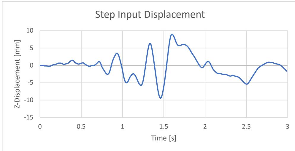
Figure 7. Step input response over a 1 cm bump at 0.47 m/s.
