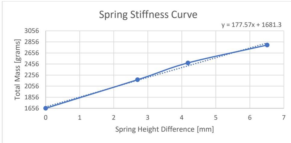
Figure 5. Spring stiffness curve
