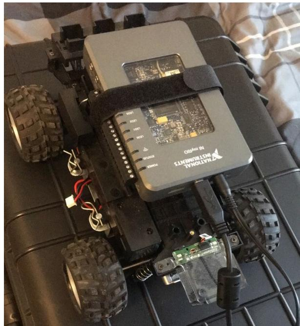
Figure 2. NI MyRIO with onboard accelerometer.
